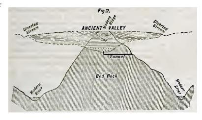
the hillside to tap the bed and drain off the water, and to serve as a tramway for delivery to the surface. The auriferous gravel is excavated, carried to the surface, and dumped on to a sloping floor at the mouth of the tunnel, and washed thence through a line of sluices, provided with riffles to catch the loose particles of gold—the gold dust.
