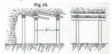
The excavation is partly filled in or walled up with large bowlders to prevent extensive caving.
